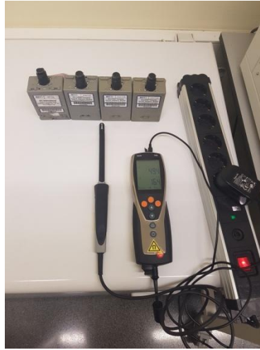
The four microPEM tested and the Testo thermohygrometer used in the experiment.
