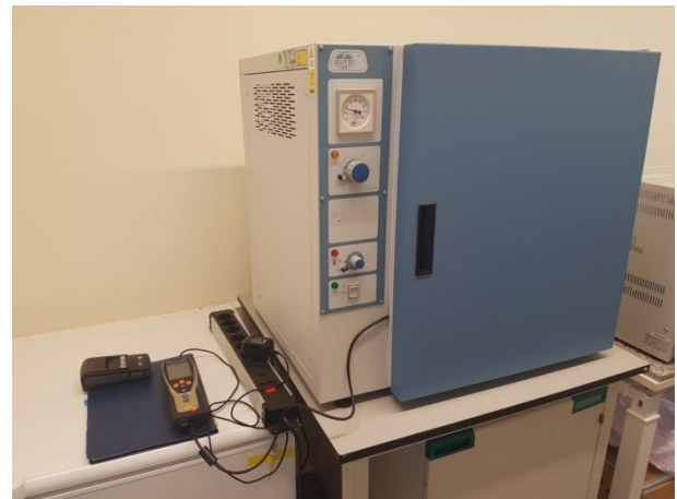
Heater used in the experiment. Left picture is with the two doors open (glass door and main door). Right picture is with the door closed (temperature probe was inside the heater but monitor was kept outside).
