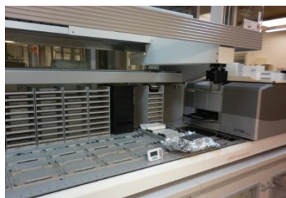
Figure 3. Tecan Microplate Reader ULTRA 384 integrated in a robotic platform (Genesis Workstation 200) that can automate the reading process.
