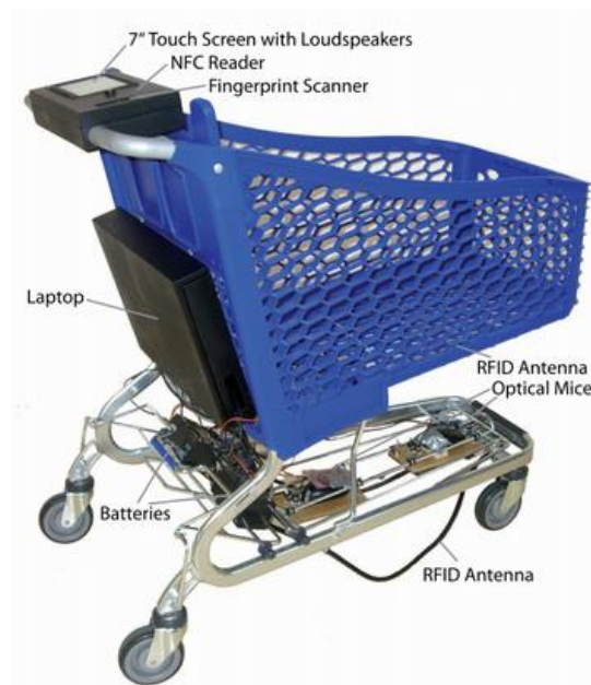
Figure 6. Trolley with 2 antennas and an optical mouse to navigate on the supermarkets (IRL-SmartCart)[2]
