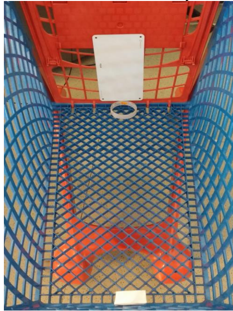
Figure 17. First test of antenna p11
