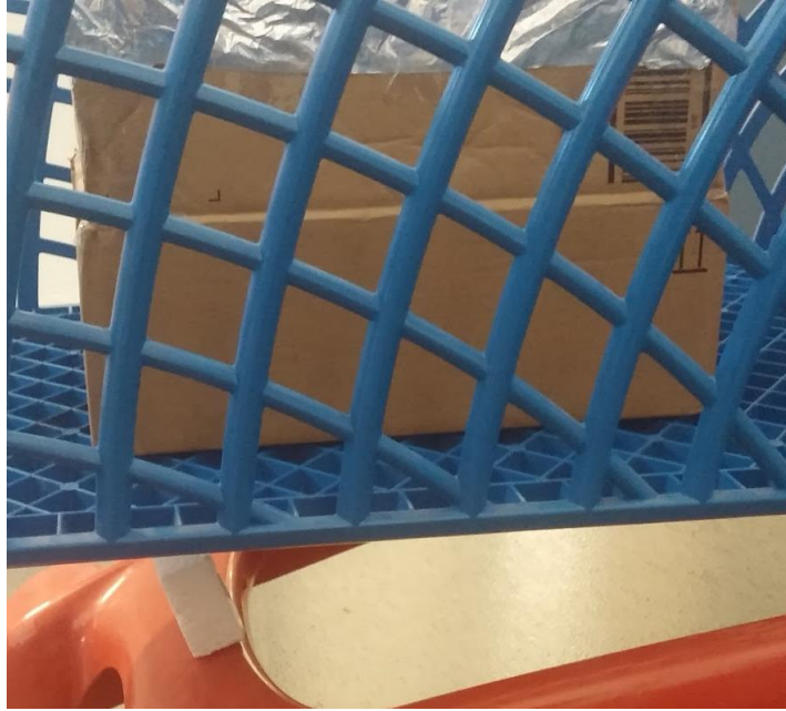
Figure 21. No detection from a tag that is under the box covered with foil
