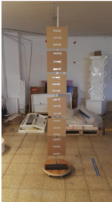
Figure 2.1. Fixed test structure of RFID tags
