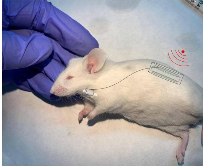
Fig. 3. Global sketch of the vagus nerve stimulation system whose development starts in this BT. Cuff electrodes are planned to deliver stimulation in the cervical region of the nerve, while the generator is expected to be placed in the back. Stimulation will be controlled with an external IR system.
