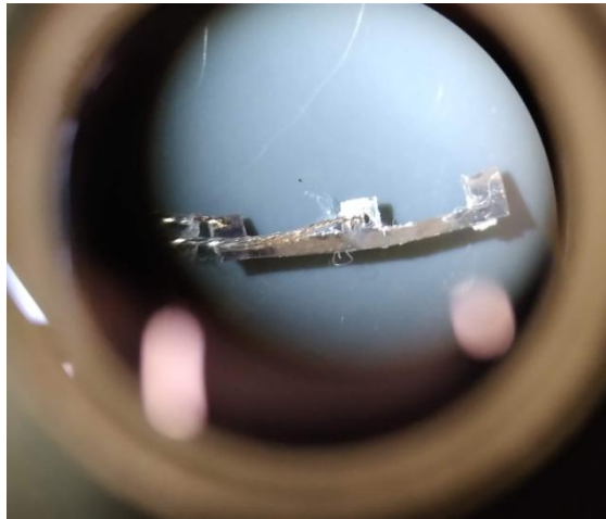
Fig. 21. Stainless steel wires soldered to the electrodes.
