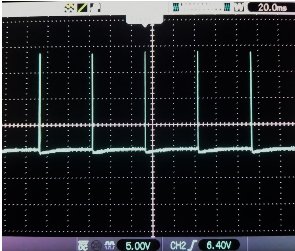
Fig. 17. Voltage at the output 12k\Omega resistance when the source is programmed to deliver 500\ \mu s pulses at a 20\text{Hz} frequency.
