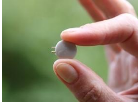
Fig. 2. Invilog Ltd. implantable wireless electrical stimulator.
