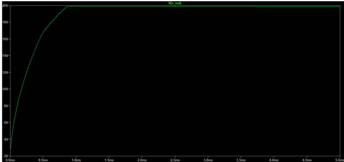
Fig. 11. Simulation of the behaviour of the LT3467 when being configured to output 20 V.
